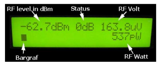
If no attenuator is used, the dBm readout goes from -63 (noise floor) to +30 dBm (1W)
