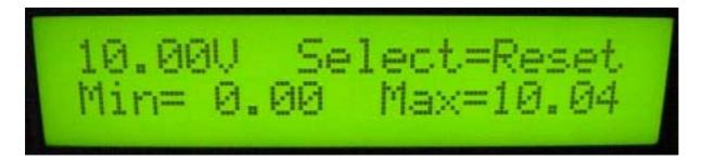
The DC voltmeter can measure from 0 to 20 volt only positive, with a resolution of 20mV. Nothing is burned if input is reversed, it just cannot measure!
