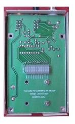
PM1A in a metal case. LEDs fitted on back of the board.
