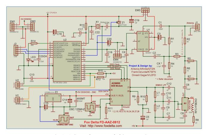
The circuit diagram (FD-AAZ-0912) of the SWR-Analyzer
