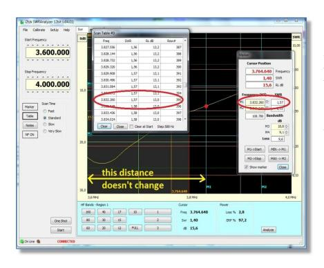
It can be seen that the values and the Scan Table & Marker windows reflect the measured values associated at the frequency, where the M1 marker intersects the graph, i.e. M1 maker is in the same position on the screen in both figures.
