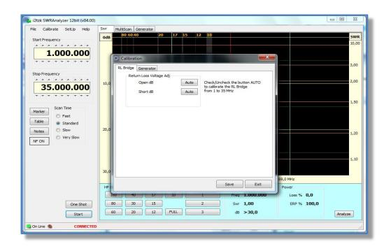
When the "Open circuit" checks are successfully completed the button [Auto] turns green to indicate that this step has been successfully executed.
