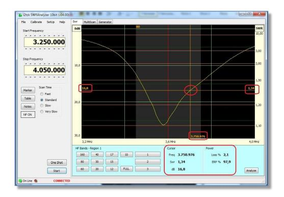
BY moving the mouse over the graphic, two lines (vertical and horizontal) will appear that follow the graphs curve and will continually display the measured values at any position the mouse stops at.
