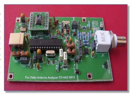
Generally speaking, the higher the DC voltage output, the worst the impedance mismatch is.
