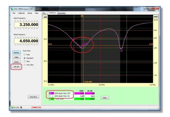
The figure has a red circle highlighting the effect of noise on the antenna return loss measurement.
