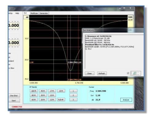
Click on the [Analyze] button to display the resonance parameters in the pop-up window.
