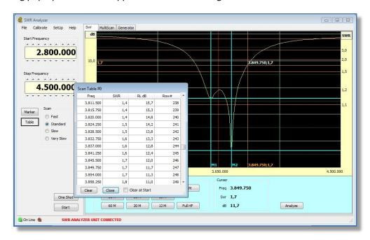
For a more detailed analysis the Data Table can be exported using the Windows menu bar [File] [Export] and then imported into any spread sheet as a CSV (Comma Separated variable) file e.g. MS Excel or other that can read the CSV format.
