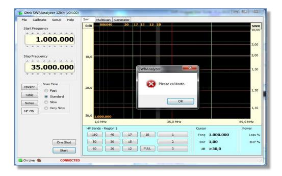
The bridge calibration requires two simple steps: a calibration of the BNC connector with an Open and Short circuit. (A paper clip cut in half is convenient way to create the short circuit)
