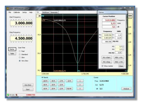
When filter has been tuned, select the [SWR] tab and select the band the filter works in, and click on [One Shot] to view a plot of the filters return loss.
