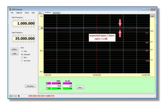
The dB difference of 2 horizontal traces across the whole HF bands, measures the Open/Short ratio.
