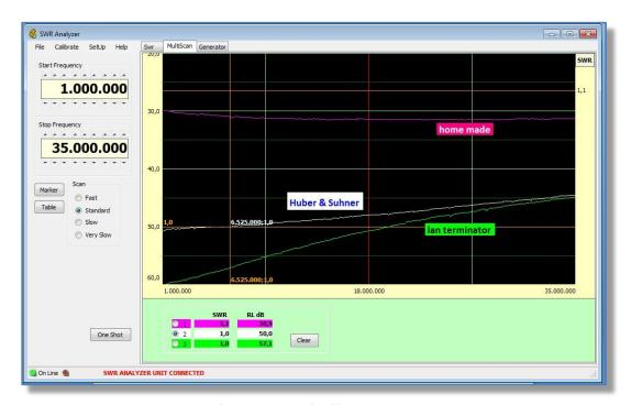
Figure above shows the results for a variety of different terminations.
