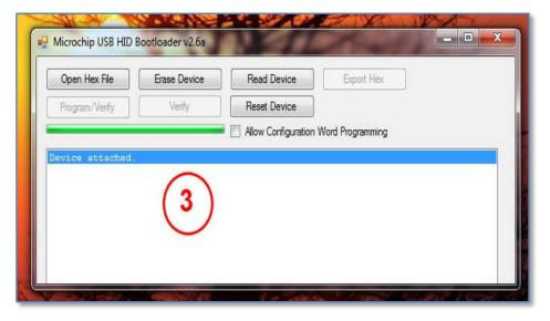
After a while, the Microchip Bootloader software identifies the Analyzer is ready to program and a green line appears along with the message "Device attached" appears and the programming buttons are enabled.
