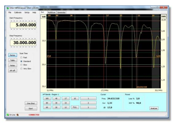
Three additional buttons numbered 1-3 are available for pre-defining custom frequency ranges. From the menu bar select [SetUp] and then in the new pop-up window select the [Generator] tab. Define each of the three buttons by using the up/down arrows. The number boxes may be edited to show the names (12 characters) of each button e.g. button 1 could be named "40m-30m"
