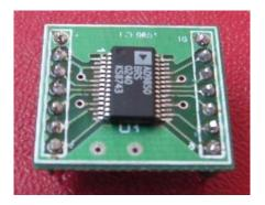
Kits are supplied with AD9850 (or AD9851) Pre-soldered on a carrier board for easy assembly. This plug-in DDS module is tested for full HF range before including with kits.
