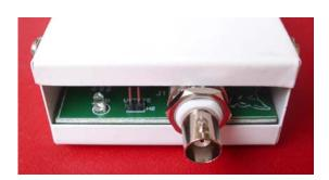
Like on AAZ0912 Boards, Front Side of AAZ-0713A has a BNC connector, Activity LED and an Update header.
