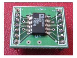
DDS: AD9850 is supplied with kits as a Pre-Soldered and fully tested for 0 to 35MHZ range. Solid Pin Header Male/Female are supplied for easy removal of this module in case of damage.
