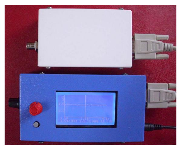
A male to Male D9 cable is required for interconnection of Graphic CPU and AAZ-0713A boards.
