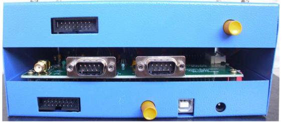
Bottom Push switch = USB / DC12V (+Battery) TOP Push Switch = Battery ON Bottom FRC16 = COMM Connector. Top FRC16 = Bluetooth connector **Basic design concept of SWM5:**
