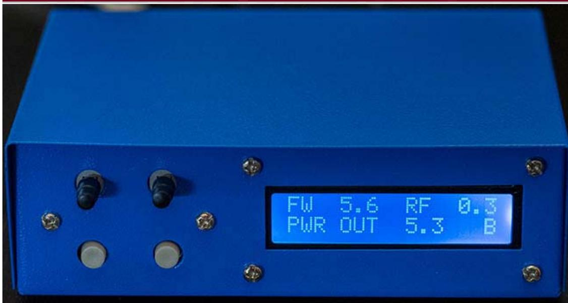
*Front Panel Switches: Power ON/OFF (Left) Battery/USB Power (Right)*
