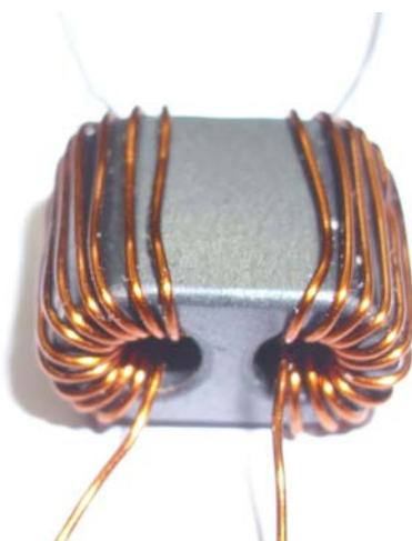
Wind 10 to 11 turns of supplied copper wire.
