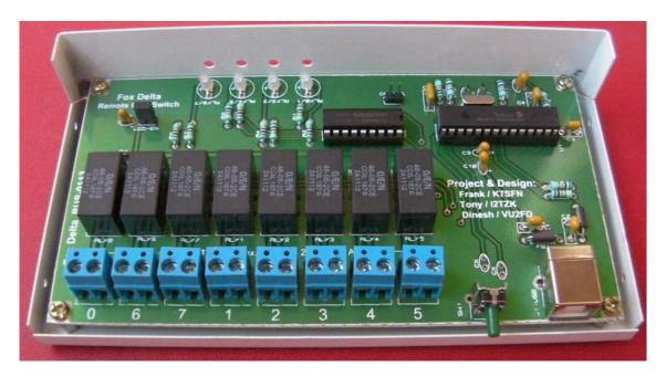
The FoxDelta RUS-1112 Remote USB Switch utilizes an 18F2550 PIC, connected to a ULN 2803 Buffer, driving eight small PCB 5V Relays. Each Form A Relay circuit is rated for 30vdc/2A and 120vac/1A. Power is supplied by your computer's USB Port. No external power source is required.
