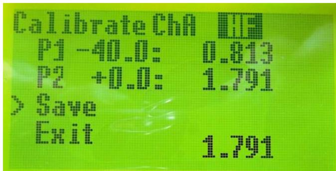
19. Press and hold the “Red” Button to Save the calibration data, and return to the previous display screen (Calibrate Selection Screen). The “>” should be next to the “EXIT” selection.
