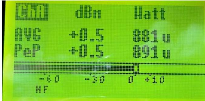
21. You can step thru the screens using the two “White” Buttons. If you are still applying a 0 dBm signal from your signal generator, it should be displayed on the PM5 screen.
