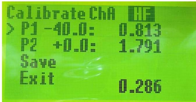
10. Apply a -40dBm signal at 10 MHz (or any HF Frequency) from an external signal generator or source.
