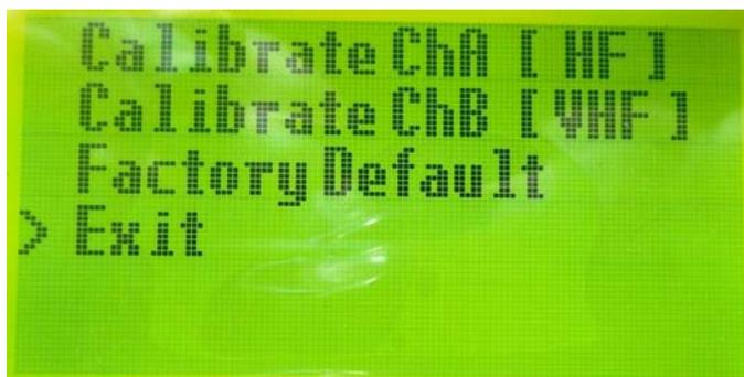
20. Press and Hold the “Red” Button to exit the Calibration Mode and return to the Measurement Display screen.
