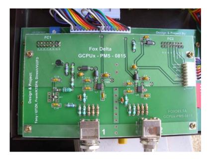
PM5 board is supplied with AD8307 and A1 (ERA3SM) pre-soldered on board. Assembly is simple and only few components to solder.
