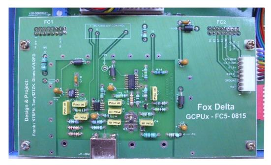
Component RX is not required when used with GCPUx Main Board. If you wish to use FC5 board for your own project, please add RX as 470K resistor.
